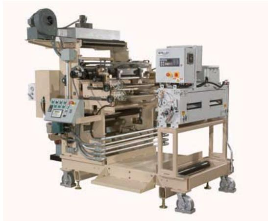
The **K-Series** line of flexo stack presses is designed for narrow to mid (**10" – 60" wide**) webs. These presses can be part of an existing line, or they can include an unwind, drying/curing system and rewind for off-line operation. They can achieve speeds up to 1000 fpm with a typical repeat range of 14" – 28".
