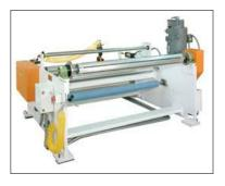
RETROFLEX custom designs unwinds and rewinds to fit your particular applications. These units can be simple single position, single spindle units or turret type systems complete with automated splicing and transfer capabilities.
