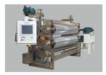
Retroflex coaters can operate in-line with your existing equipment lines or they can be equipped with various components such as an unwind, dryer and rewind for off-line operation. Reverse angle and trailing doctor blade systems as well as fountain type fluid metering systems are available for the application of waterbased and UV fluids.
