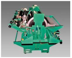
The Fox-Series line of CI presses is designed for mid to wide (60" - 100" wide) webs. These presses can be part of an existing line, or they can include an unwind, drying/curing system and rewind for off-line operation. They can reach speeds over 2500 fpm with a typical repeat range of 36"-48".
