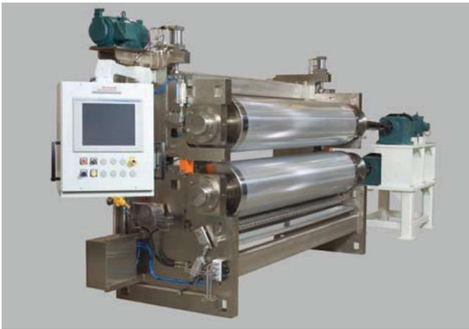
Retroflex single and two side coaters are available in direct gravure, offset gravure and flexographic designs. Coaters can be designed for operation at speeds up to 3750 FPM with web widths of 10" up to 150". Two side coaters can apply fluid to both sides of the web simultaneously. Temperature controlled rolls and doctor blade systems are available for specialty fluids such as wax, lotions, or anti-bacterial solutions.
