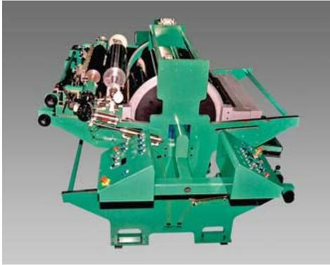
The Fox-Series line of CI presses is designed for mid to wide (60" - 100" wide) webs. These presses can be part of an existing line, or they can include an unwind, drying/curing system and rewind for off-line operation. They can reach speeds over 2500 fpm with a typical repeat range of 36"-48".
